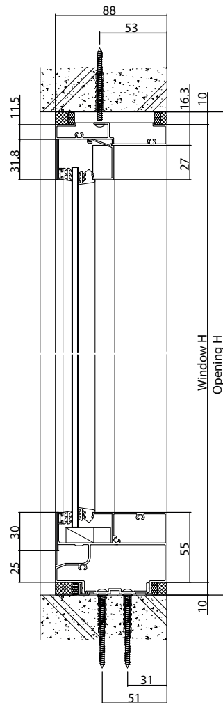
Vertical section: Single fixed window
